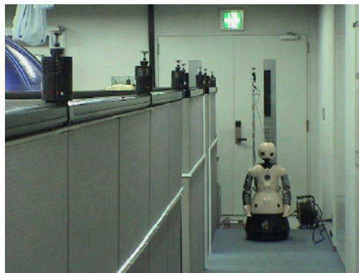
Fig. 1. The humanoid robot Eveliee and the DVS installed in the environment
