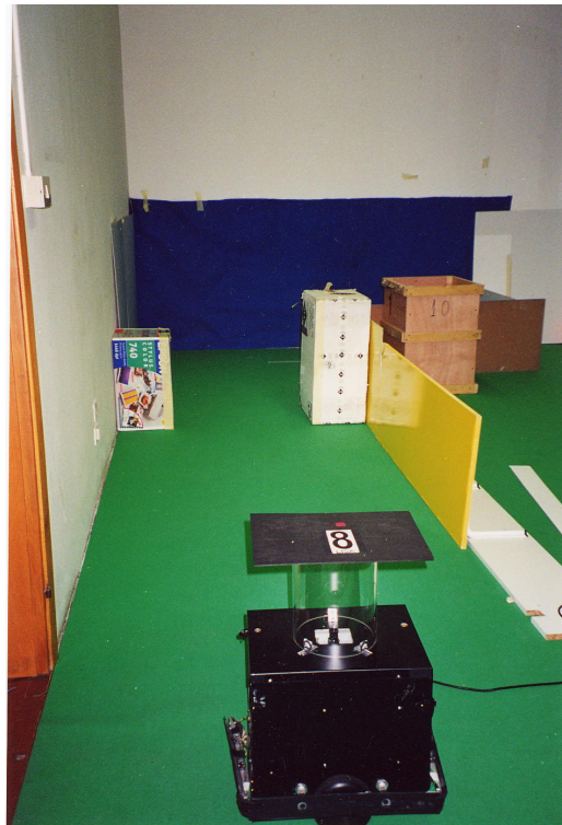
Figure 5.5: The experimental set-up. This is the corridor where the experiments were conducted. The two boxes represent a door. On the right, behind the wood box there is the turn of the corridor.
