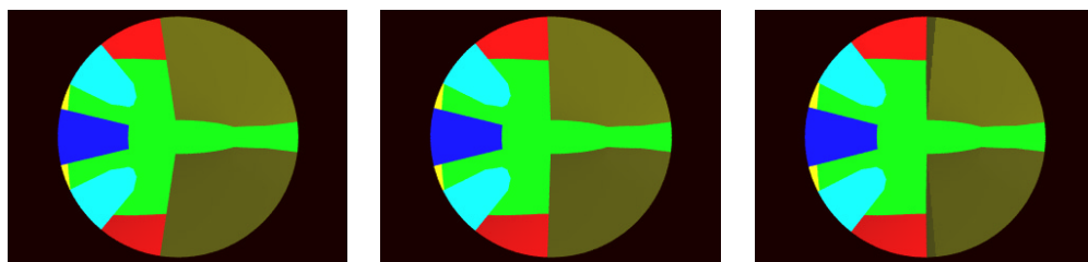
Figure 2.6: The simulation of an edge going to be occluded. In the first frame, the edge between the yellow corridor boxes and the red walls are clearly visible. In the second frame, they are just visible. In the third frame, they disappeared.
