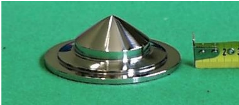
Figure 2: The mirror with the custom profile we designed
