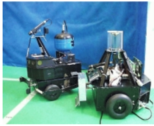
Figure 1: (Left) A close view of the vision system of Nelson. On the left, the perspective camera. In the middle, pointed up-ward the omnidirectional camera. (Right) A close view of two of our robots. Note the different vision systems.
