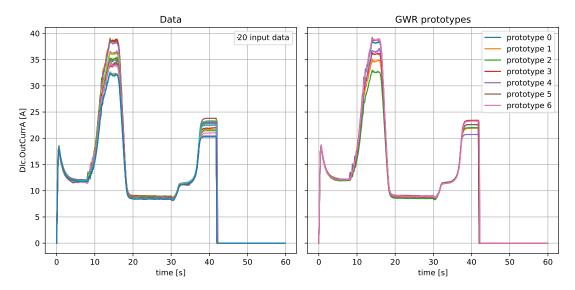
**Figure 4:** The left part of the figure shows the values of an engine's current consumption in a particular session. These values have been used to create the reference dictionary depicted in the right part of the figure, using GWR.
