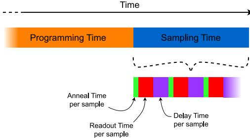
Fig. 1: The quantum annealer access time split in several steps.
