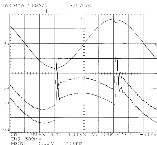
Fig. 7. Load step variations. Output voltage (channel 3) 100 V/div, current reference (channel 2) 10 A/div, and actual current (channel 1) 10 A/div; horizontal 2.5 ms/div.
