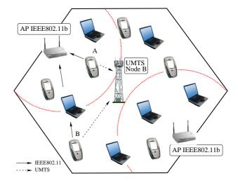
Figure 1: An example of heterogeneous wireless network.
