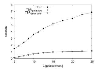
Figure 4: Average end-to-end (nodes  $\rightarrow$  APs) packet delay.
