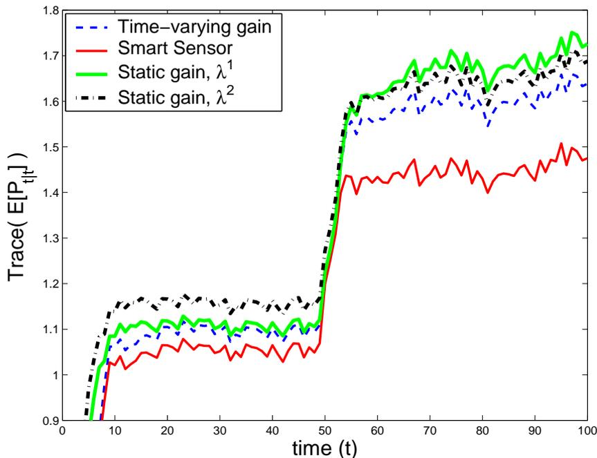
Fig. 9. Time series of trace of trace of empirical error covariance  $P^{emp}(t) \cong \mathbb{E}[P_t|t]$  averaged over 1000 Monte Carlo runs for four different estimators under the same conditions. The packet delay arrival probability distribution changes from  $\lambda^1$  to  $\lambda^2$  at time  $t = 50$ . The filters with static gains are optimized for  $\lambda^1$  and  $\lambda^2$ .
