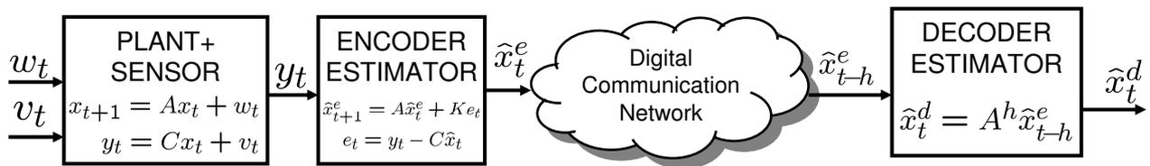
Fig. 6. Smart sensor with state estimator at encoder site before transmission.
