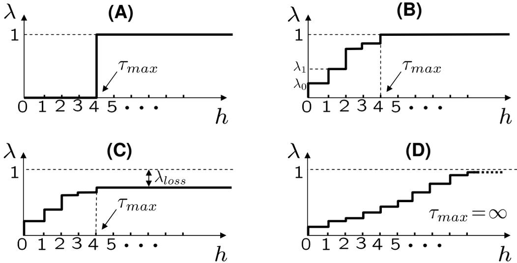
Fig. 5. Probability function of arrival process  $\lambda_h = \mathbb{P}[\tau_k \leq h]$  for different scenarios: deterministic packet arrival with fixed delay (A); bounded random packet delay with no packet loss (B); bounded random packet delay with packet loss (C); unbounded random packet delay with no packet loss (D).
