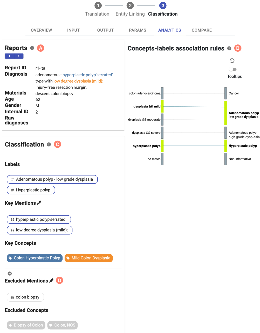
Figure 5: SKET X Analytics tab for the classification phase: (A) reports section to select the current report via left/right buttons; (B) SKET rules for determining the labels visualized with a Sankey diagram; and, (C) list of labels, mentions, and concepts determined by SKET. Each concept and the related mentions are highlighted with the same color in (A) and (C). The Sankey diagram highlights the relevant rules by clicking/hovering on a specific label. On the left side of the Sankey diagram are reported the rules triggers . If one or more concepts satisfy a rule trigger, then the related label is highlighted on the right side of the Sankey diagram and also listed in (C). The mentions and concepts involved in the classification task are the key mentions/concepts (C), while the excluded ones are reported in (D).
