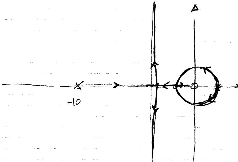
$$2) (s-1)^2(s+p) + s = (s^2 - 2s + 1)(s+p) + s = (s^2 - 2s + 2)s + (s-1)^2 p = 0$$
