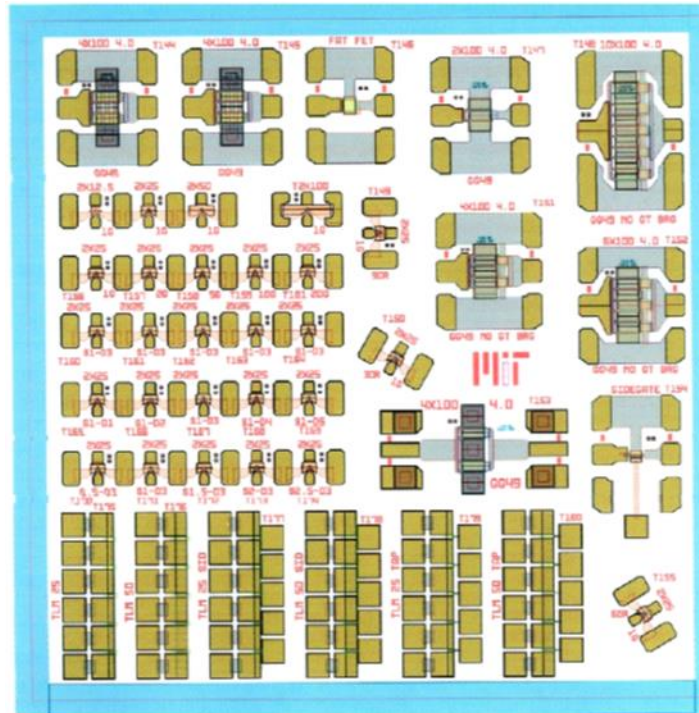
Fig. 34 : Reliability test structure adopted by MIT (J. Joh and J.A. del Alamo, tutorial notes of ESREF 2009, http://www-mtl.mit.edu/~alamo/pdf/2009/RC%20160%20slides.pdf , [132])
