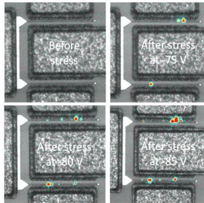
Fig. 5: EL microscopy images of a representative HEMT sample. Images were taken at V_G = 10 V (with V_S = V_D = 0 V) after each step-stress.
