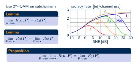
In the high SNR limit, any rate that is achievable by independent Gaussian inputs is also achievable by uniform QAM inputs with sufficient cardinality
