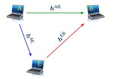
$h = [h_0, \dots, h_{N-1}]$ : channel fading coefficients (e.g., impulse response, frequency response, channel matrix entries)
