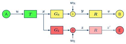
• instance of MIMO Gaussian wiretap channel (MIMOME) with  $H_{\rm R} = RG_{\rm R}T$  diagonal, and  $H_{\rm E} = RG_{\rm E}T$
