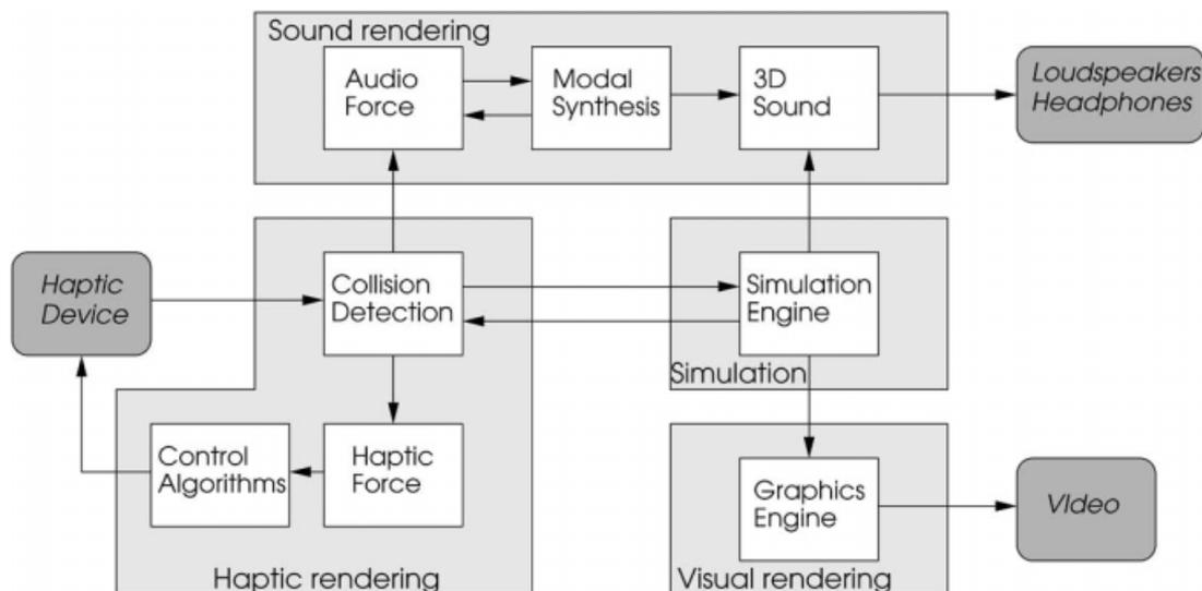
Figure 1. An architecture for multimodal rendering of contact interactions. Adapted from Figure 3 in Reference [25].
