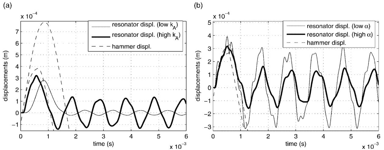
Figure 2. Examples of transient attacks obtained from the impact sound model: (a) short versus long initial bumps, obtained by varying the force stiffness  $k_A$ ; (b) single versus multiple contacts obtained by varying the exponent  $\alpha$ .
