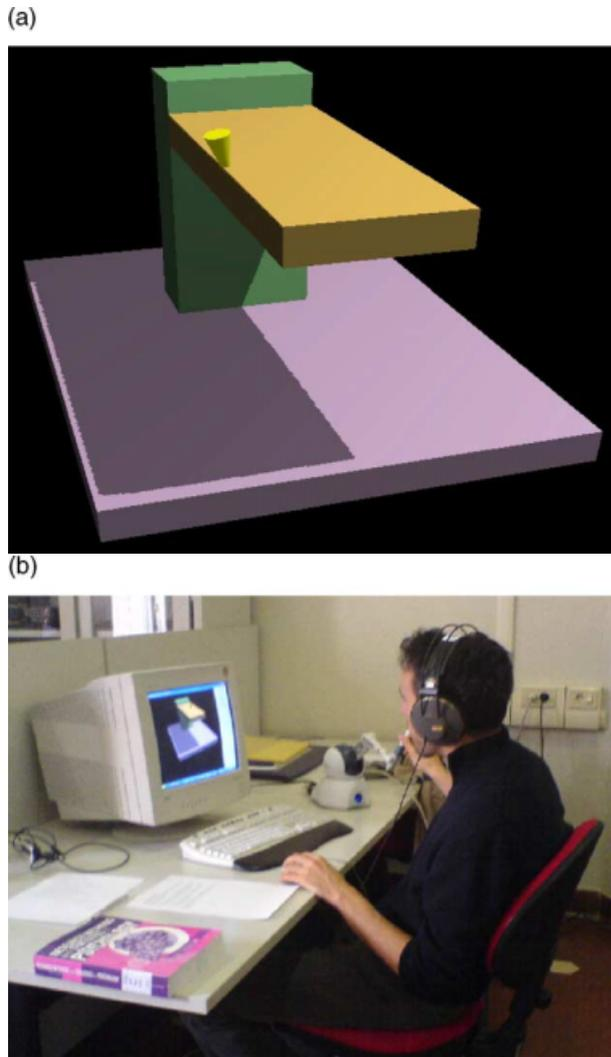
Figure 4. Experimental procedure: (a) interactive graphic display presented to the subjects (the small cone represents the tip of the Phantom<sup>®</sup> Omni<sup>™</sup> stylus); (b) experimental setup.
