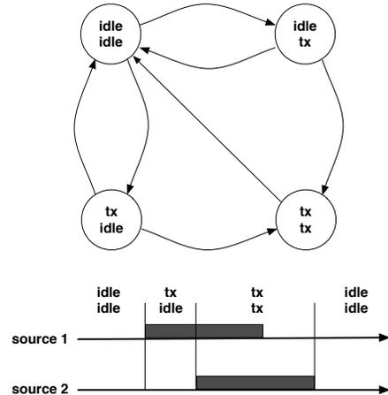
Figure 9. State space diagram and example of network state pattern for a network with 2 primary sources.
