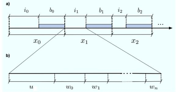
Figure 1. a) Alternate renewal process of the primary source, b) characterization of the idle time.
