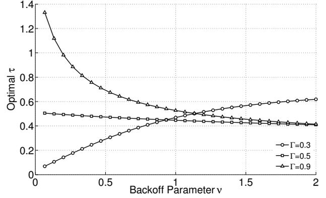
Figure 7. Optimal transmission duration  $\tau$  of the secondary user as a function of the backoff parameter  $\nu$ .
