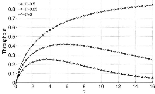
Figure 4. Throughput of the secondary user as a function of the duration  $\tau$  of its transmission period.
