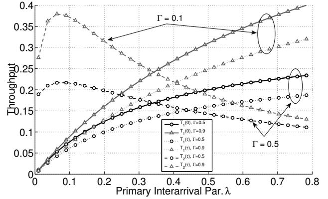
Figure 8. Throughput of the primary ( $\mathcal{T}_1$ , dotted) and secondary ( $\mathcal{T}_2$ , dashed) users as a function of the traffic intensity of the primary  $\lambda$ .
