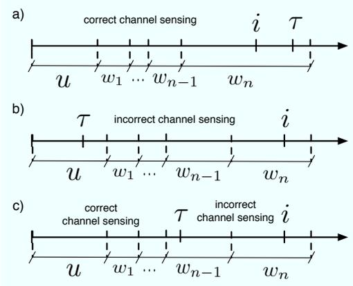
Figure 3. a) the transmission time  $\tau$  is larger than  $i$ , b) the transmission time  $\tau$  is smaller than  $i$  and the interarrival time  $u$  is larger than  $\tau$ , c) the transmission time  $\tau$  is smaller than  $i$  and the interarrival time  $u$  is smaller than  $\tau$ . In the cases a and b, the figure refers to the nontrivial case in which  $u \leq i$ .
