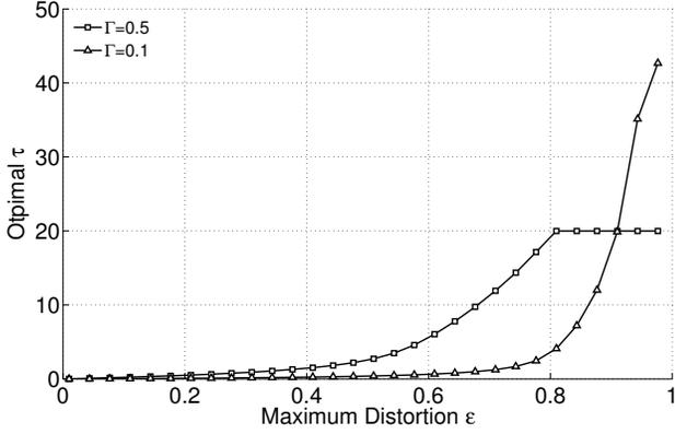
Figure 6. Optimal transmission duration  $\tau$  of the secondary user as a function of the primary quality constraint  $\epsilon$ .
