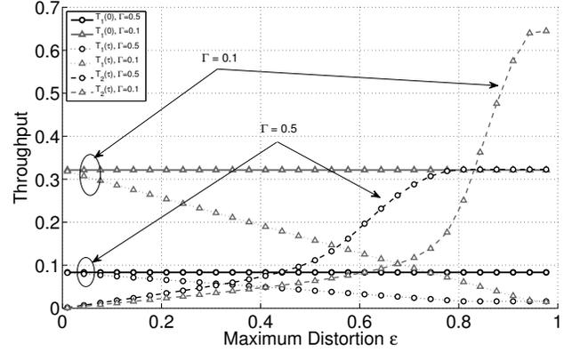
Figure 5. Throughput of the primary ( $\mathcal{T}_1$ , dotted) and secondary ( $\mathcal{T}_2$ , dashed) users as a function of the primary quality threshold  $\epsilon$ .
