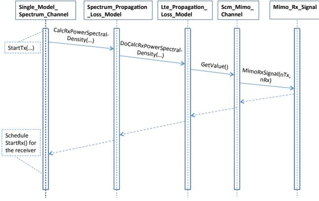
Fig. 2: StartTx method for the transmitter
