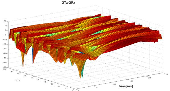
(b) Channel gain between antenna pair Tx = 2, Rx = 2
