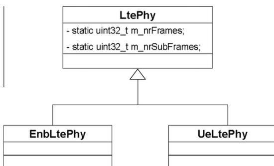
Fig. 4. UML class diagram for the PHY layer in ns-3 LTE.
