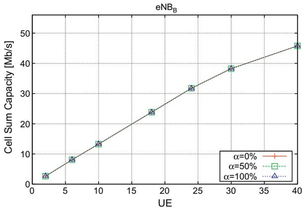
Fig. 9. Cell sum capacity for  $eNB_B$  versus the number of UEs in cell B in the asymmetric load scenario.
