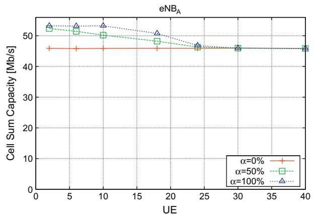
Fig. 8. Cell sum capacity for  $eNB_A$  versus the number of UEs in cell B in the asymmetric load scenario.
