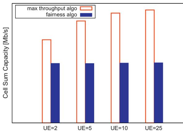
Fig. 6. Comparison of the cell sum capacity for the *max throughput* and the *fairness* allocation algorithms, with a sharing percentage of 100%.
