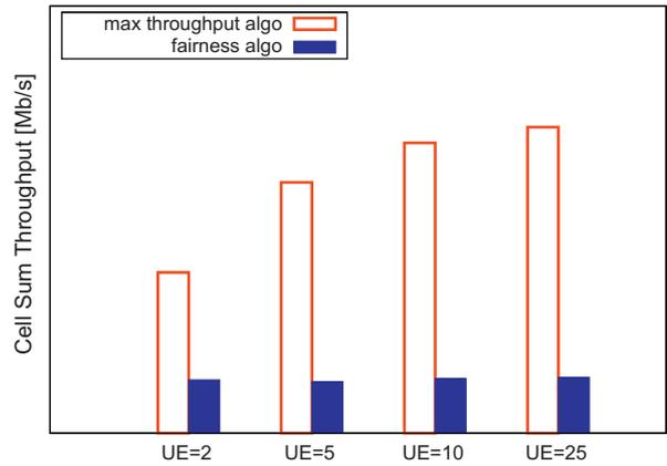
Fig. 7. Comparison of the Cell Sum Throughput for the *max throughput* and the *fairness* allocation algorithms, with a sharing percentage of 100%.
