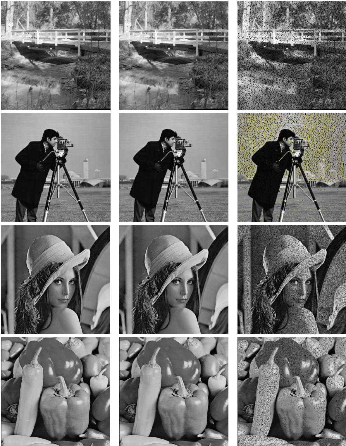
Figure 1: Compression and reconstruction of images. The original is on the first column, next to its reconstruction by interpolation of two closest solid pixels. Black dots used in the figures of the last column are used to display the distribution of the don't care characters. Compression of "Bridge" at 1/4 and 1/3 (shown here) './char densities yields savings of 6.49% and 17.84% respectively. Correspondingly, 0.31% and 12.50% of the pixels differ from original after reconstruction. The lossy compression of Camera at 1/4 './char density saves 11.60% over GZip. Only 6.67% of pixels differ from the original after reconstruction. Gains by "Lena" at 1/4 and 1/3 (shown) './char density are respectively of 10,13% and 25,33%, while interpolation leaves resp. 3,85% and 10,13% differences from original. For "Peppers" (last row), the gains at 1/4 and 1/3 (shown) './char densities were respectively 14,09% (5,56% the corresponding difference) and 25,30% (16,67% diff).
