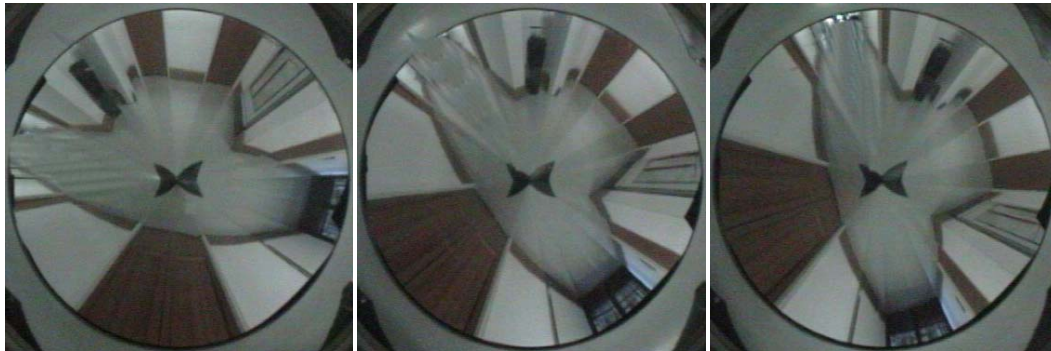
Fig. 8. The sequence of images acquired by the omnidirectional camera of the robot while it turns on the spot
