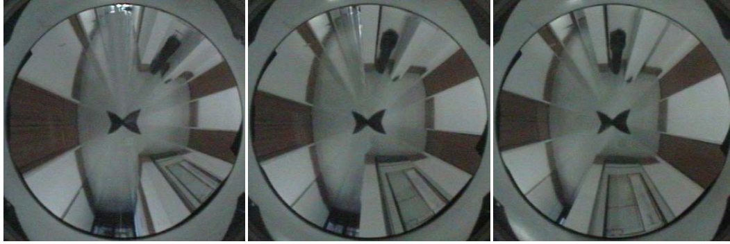
Fig. 7. The sequence of the robot passing through a door. In the first frame, the posts of the door are not yet at 180 deg. In the second frame, they are at 180 deg. In the third, they are not longer at 180 deg.
