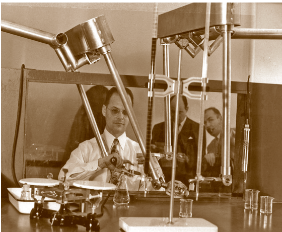
Fig. 31.2 Raymond C. Goertz used electrical and mechanical teleoperators in the early 1950s to handle radioactive material. (Courtesy Argonne National Labs)
