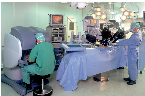
Fig. 31.7 Intuitive Surgical Inc. makes the da Vinci telerobotic system, which is used in minimally invasive surgery. (Courtesy ©2008 Intuitive Surgical, Inc.)
