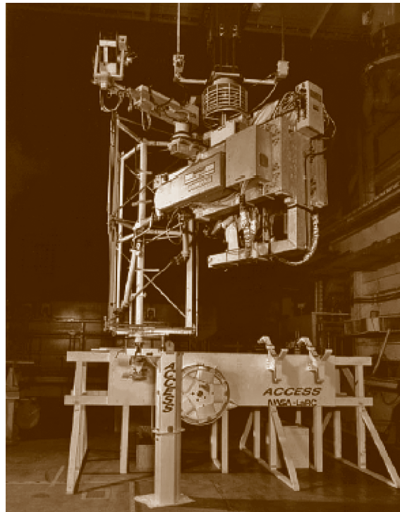
Fig. 31.3 The telerobotic system CRL Model M2 is used to verify the assembly of space truss structures (1982). (Courtesy of the Oak Ridge National Laboratory)
