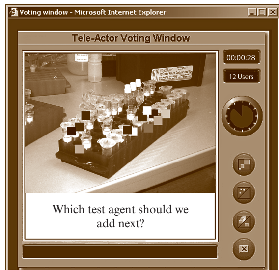
Fig. 32.11 Spatial dynamic voting interface for the Tele-Actor system [32.41]: the spatial dynamic voting (SDV) interface as viewed by each user. In the remote environment, the Tele-Actor takes images with a digital camera, which are transmitted over the network and displayed to all participants with a relevant question. With a mouse click, each user places a color-coded marker (a votel or voting element) on the image. Users view the position of all votels and can change their votel positions based on the group's response. Votel positions are then processed to identify a consensus region in the voting image that is sent back to the Tele-Actor. In this manner, the group collaborates to guide the actions of the Tele-Actor
