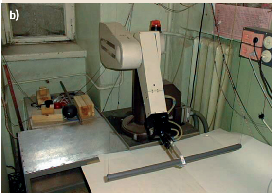
Fig. 32.10a,b A web-based teleoperation system that allows robot to capture a fast-moving rod [32.27] (a) User interface and (b) system setup
