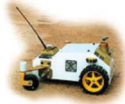
Image 1 – The Sahabot 2 records visual reference points and navigates with the help of sensors which analyse the polarization of the light.
