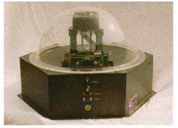
Figure 6.15: Denning Branch International Robotics (DBIR) can see *active targets* at up to 183 meters (600 ft) away. It can identify up to 32 active or passive targets. (Courtesy of Denning Branch International Robotics.)
