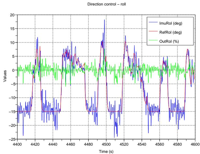
**Fig. 8.** Direction control: roll reference from the yaw controller, actual roll and elevon command
