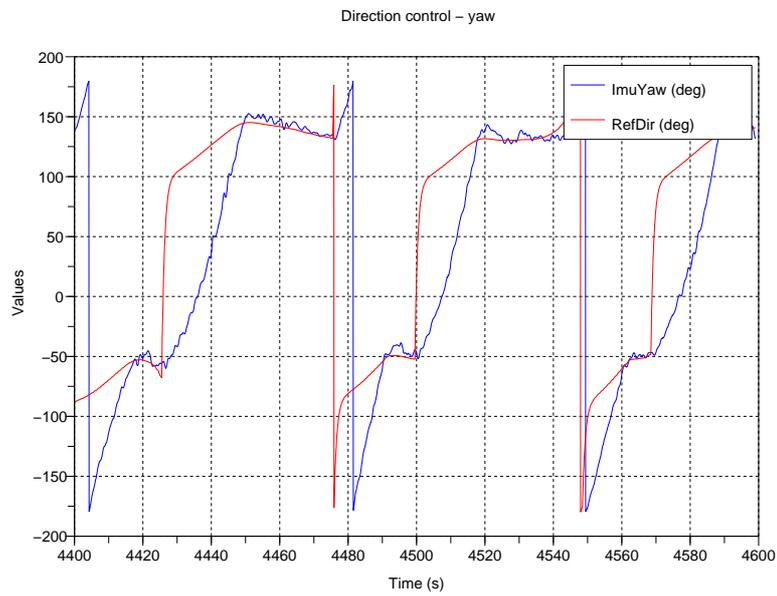
**Fig. 7.** Direction control: reference from the heading control and actual yaw
