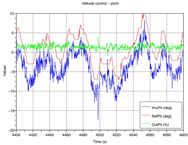
**Fig. 6.** Altitude control: desired and actual pitch; elevon command
