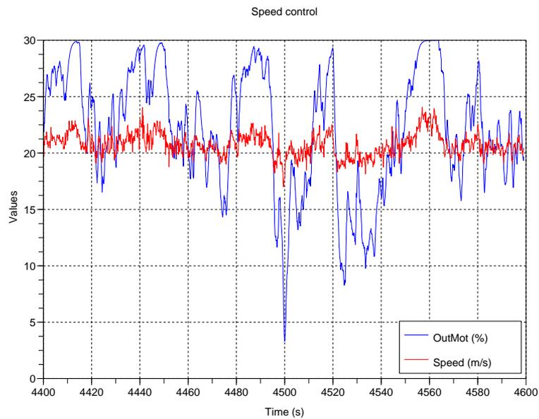
**Fig. 4.** Performance of the speed control loop: set point 20 m/s. Actual speed and motor command
