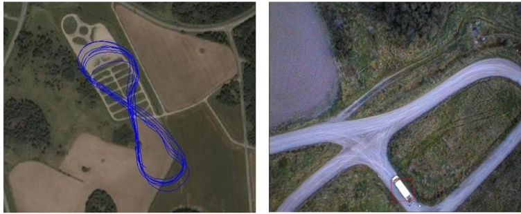
Fig. 5. On the left picture is displayed the MAV's flight path during the ground object localization task. On the right, the ground object is automatically tracked in the image (red square).
