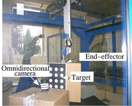
**Fig. 3.** Experimental setup : eye-to-hand configuration
