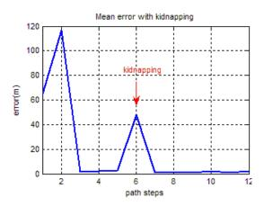
Figure 5 Results of mean error with a kidnapping situation
