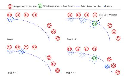
**Figure 2** - On line knowledge integration: red circles represent the previous knowledge (omnidirectional images with relative position in the environment); blu line is the robot trajectory; blu dots are MCL particles that, in case of good accumulation and low image density, bring to the knowledge update.
