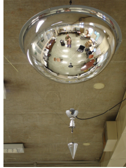
Fig. 1. The OmniEye with the spherical mirror, the camera fixed with nylon threads and the conical mass that make up the omnidirectional system.
