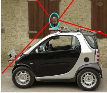
Fig. 4. Our vehicle with the omnidirectional camera (blue circle). The field of view is indicated by the red lines.
