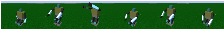
Fig. 5. Original stand-up motion replayed by the robot after kinesthetic bootstrapping. The robot does not rise too high up.
