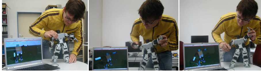
Fig. 1. A human user kinesthetically manipulates a small humanoid robot. The resulting postures are used to bootstrap a learning algorithm.
