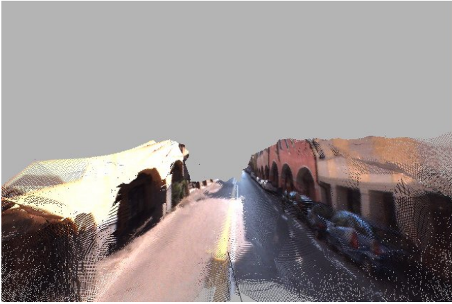
Fig. 2. A dense reconstruction of the surrounding environment obtained with the proposed method. The previous image used for this reconstruction is shown in Fig. 8(a).
