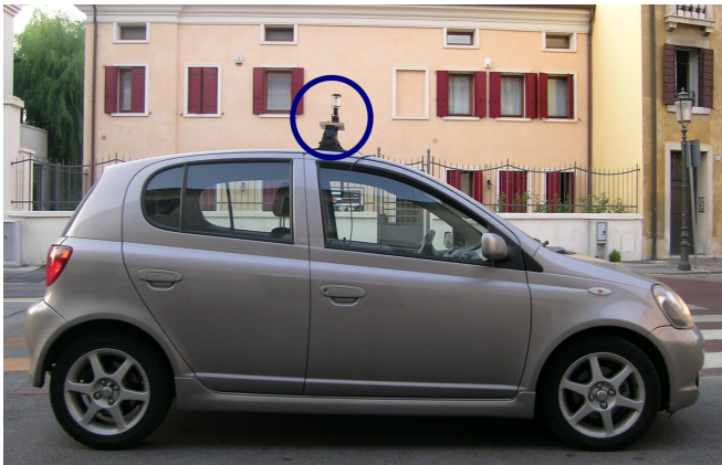
Fig. 6. The vehicle used in the experiments equipped with the omnidirectional installed on the roof (in the blue circle).
