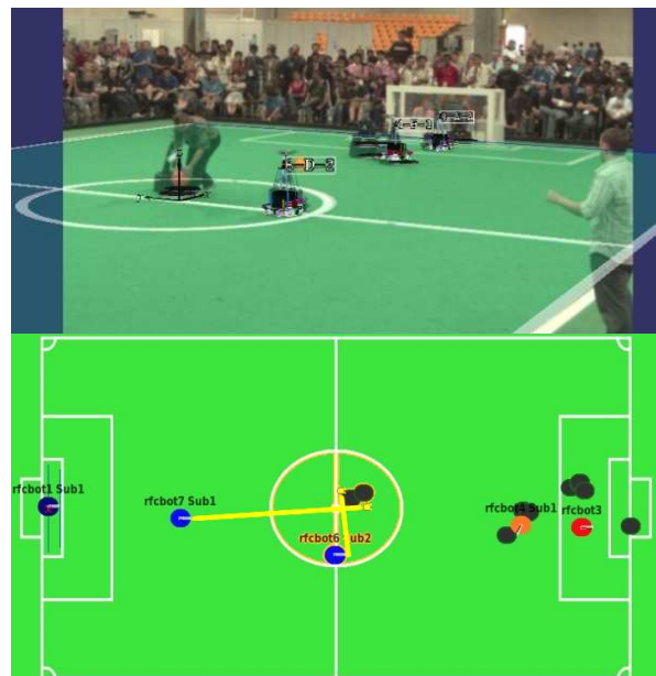
Fig. 3: Erroneous position estimation of the ball above ground during the RoboCup finals 2009 in Graz
