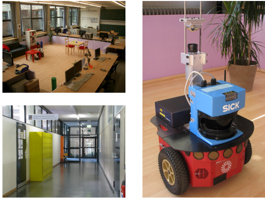
Fig. 4. The real world environment and the robot used in our experiments. The upper left image show the ZAFH laboratory, the lower left image the adjacent hallway and the right image our Pioneer 3DX robot equipped with Microspace PC and omnidirectional camera.
