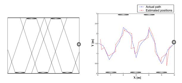
Figure 7: (Left) A sketch of the test environment with the areas monitored by every acoustic sensor. Note that in some areas of the environment there is an overlapping allowing for a simultaneous and more precise acoustic localisation of the intruder. (Right) A plot of a tracking experiment of the intruder with the ground-truth of the followed by the intruder and the estimated path.
