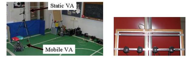
Figure 1: The sensory agent implemented: on the left, the two vision agents the static one on the tripod and the mobile one on the mobile robot; on the right, one of the acoustic agents present in the environment.
