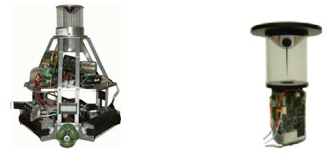
Figure 5: (Left) The mobile robot on which is mounted the mobile vision agent. This is an holonomous robot with an omnidirectional vision system where the mirror has a custom profile. (Right) A close-up view of the omnidirectional camera of the static vision agent with the hyperbolic mirror. Note the two omnidirectional sensors have very different mirrors, so they produce very different images.
