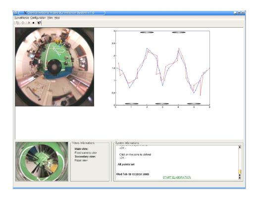
Figure 8: A screenshot of the graphical interface on the monitoring station. The remote operator is presented with the current image acquired by the static vision agent (up left), the status of the system (bottom right) and the omnidirectional image sent by the robot once the intruder is recognised by the robot (bottom left). The operator may also display the tracked path of the intruder (up right).
