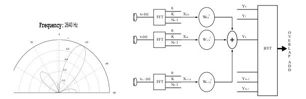
Figure 3: (Left) The reception diagram obtained for the array of microphones once beamforming is performed. (Right) A schematic representation of the beamforming algorithm.
