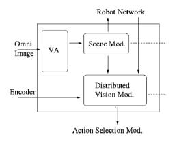
Figure 4: The architecture of the sensor fusion module.
