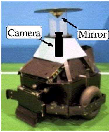
Fig. 10. The new robot (Nelson) with its omnidirectional sensor.
