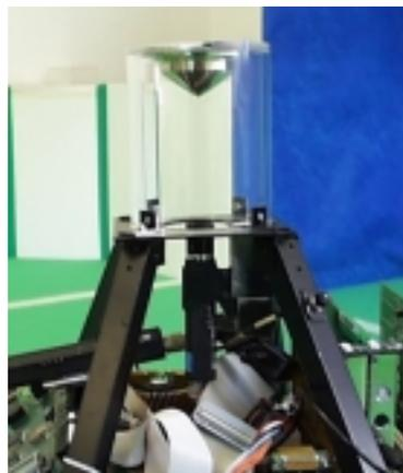
Fig. 1. The omnidirectional vision sensor of the robot. Note the multi-part mirror, whose profile is depicted in Figure 11
