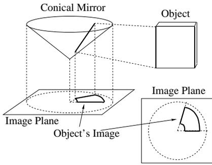
Fig. 3. The conical projection showing how a vertical line is mapped in a radial line in the image plane (adapted from Yagi).
