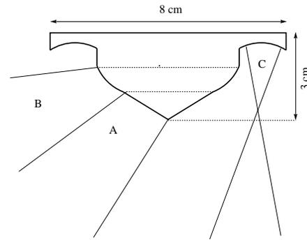
Fig. 2. A rough sketch of the mirror profile where the curvatures of the different sections are exaggerated for sake of clearness.
