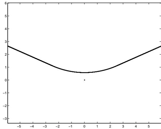
Fig. 14. The actual mirror profile of the old omnidirectional mirror.
