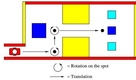
Fig. 8. The path of the robot through the virtual environment.
