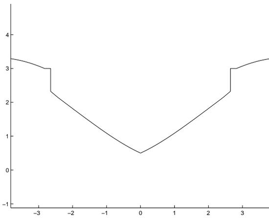
Fig. 11. The actual mirror profile of the new omnidirectional mirror designed for this application.
