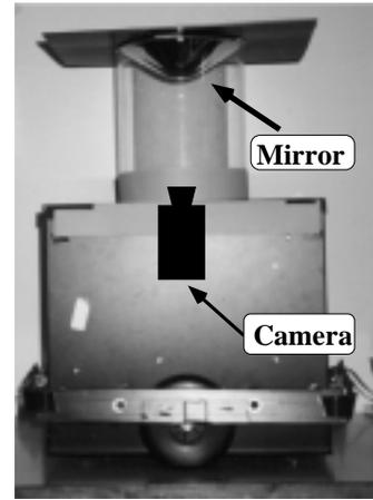
Fig. 13. The old robot (Caboto) with its omnidirectional sensor.
