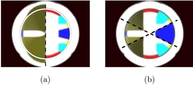
Fig. 7. (a) Event 3: the robot enters a corridor (on the left): the two edges are 180 apart (b) Event 4: the robot sees two pairs of edges at 180.
