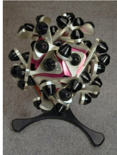
Figure 2.17: The S.O.S. sensor (Stereo Omnidirectional System) produced by ViewPLUS Inc.
