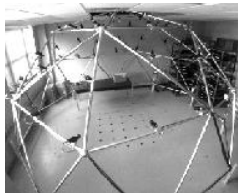
Figure 2.19: The dome for virtualising artistic or sport performance at Carnegie Mellon University.
