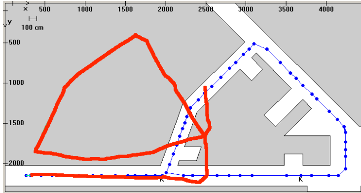
Fig. 8. The odometric data used in the experiments. Note the odometric information used by the robot is really inaccurate.
