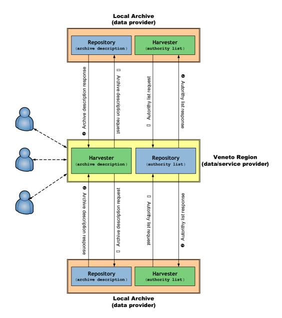
Fig. 3: Conceptual Architecture of SIAR
