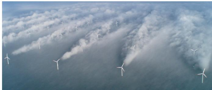
Figure 1: Wake effect on a real wind farm (Horns Rev 1): regular layouts like the one in the picture can be very inefficient for certain specific wind scenarios, resulting into a greatly reduced energy production for the whole wind farm. [Source: Vattenfall]
