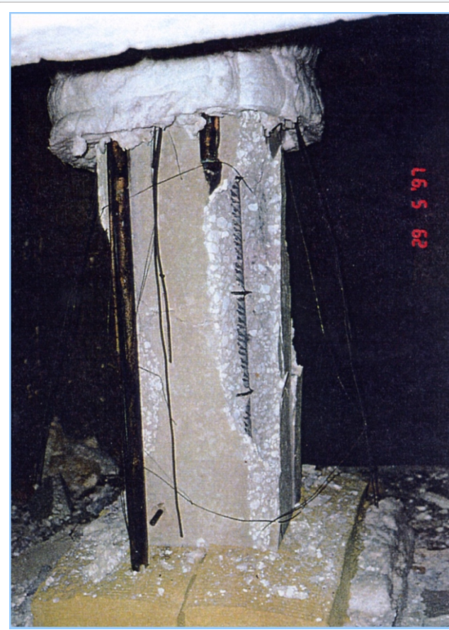
The "spalling" phenomenon in a concrete-made pillar after a simulated fire.
