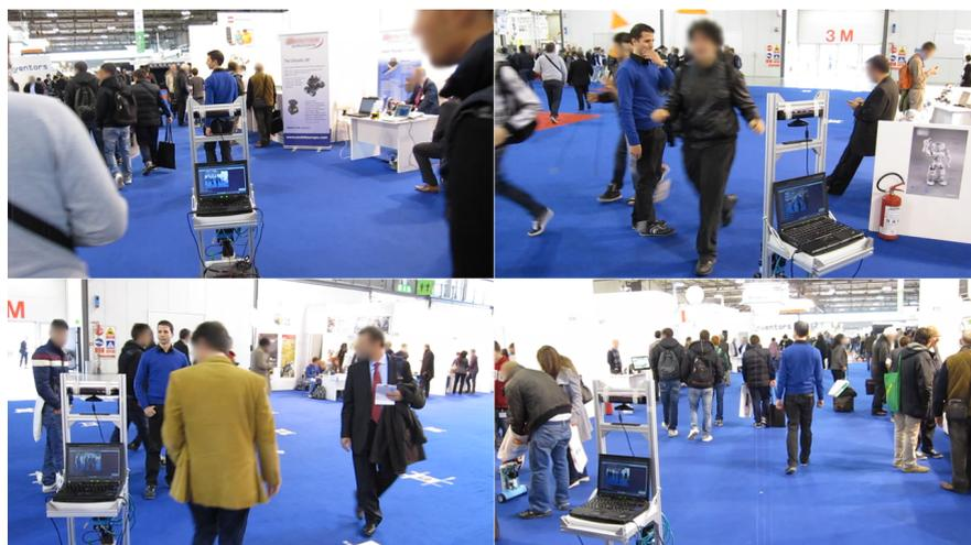
Figure 3.27: Sample images of our mobile robot following the person with the blue sweater within a crowded environment. It is worth noting that the sweater has the same color of the carpet on the floor, thus algorithms based only on color information would have easily failed.
