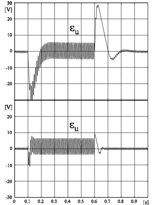
Fig. 7 - Output voltage behavior at load step change. (10%-100% of the nominal load).
