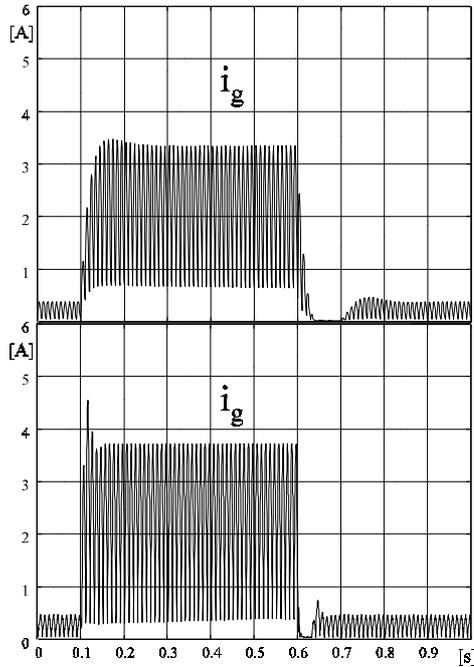
Fig.8 - Rectified input current behavior at step load change (10%-100% of the nominal load).
