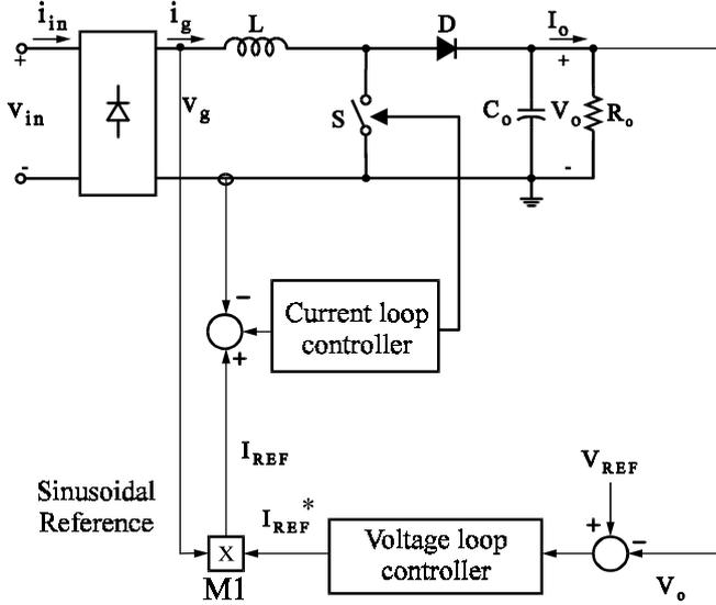
Fig. 1. Power Factor Preregulator basic scheme.
