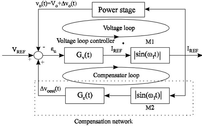
Fig. 3. Block scheme of the ripple compensation network
