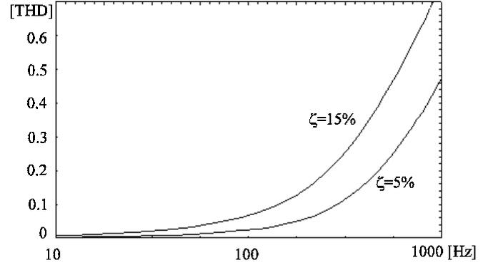
Fig. 4. Input current Total Harmonic Distortion (THD) versus voltage loop bandwidth for a specified amplitude relative error  $\zeta$  in  $\Delta v_{oest}(t)$ ,
