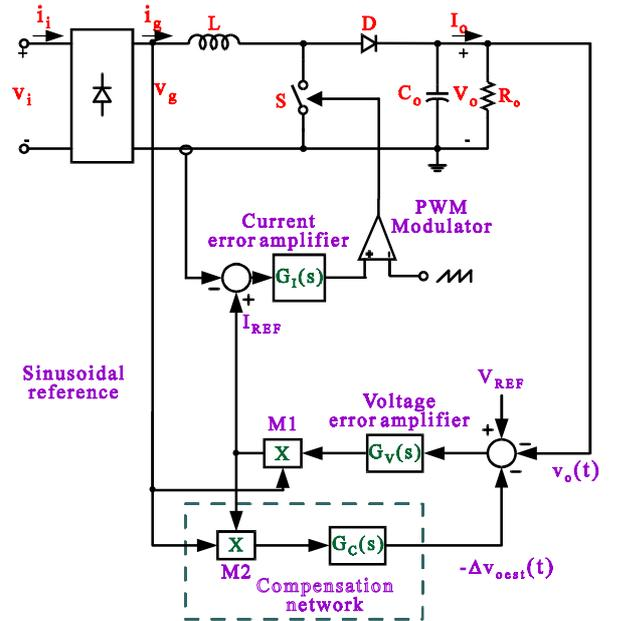
Fig. 2. Boost PFP with proposed output voltage ripple cancellation scheme.
