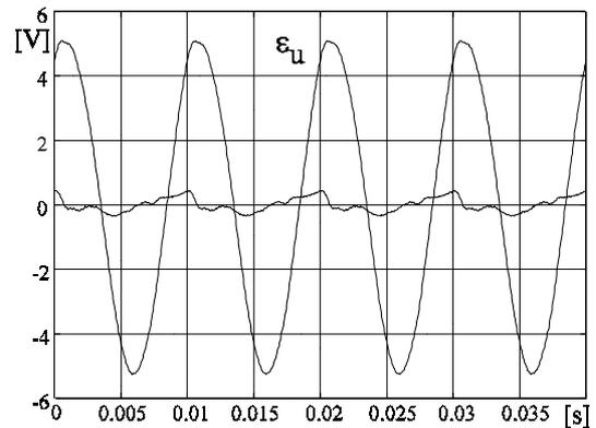
Fig. 10 - Low-frequency output voltage ripple before and after the compensation action
