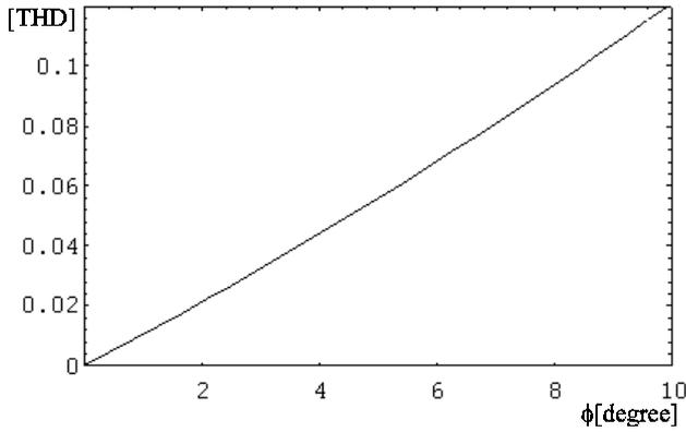
Fig. 6. Input current THD versus phase error  $\phi$  [degree] on  $\Delta v_{oest}(t)$  (voltage loop bandwidth=100Hz)
