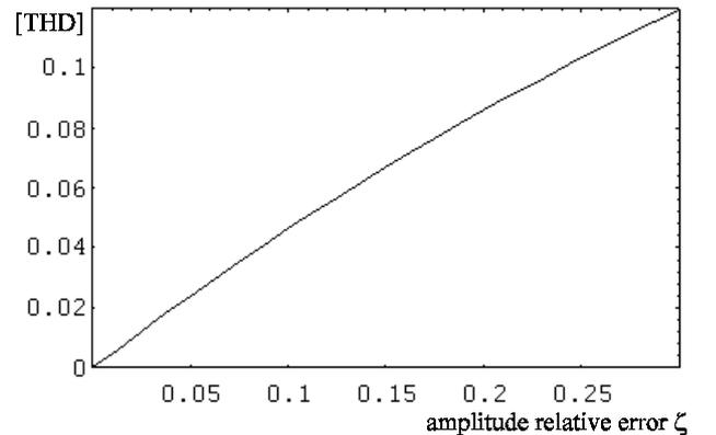
Fig. 5. Input current THD versus amplitude relative error  $\zeta$  in  $\Delta v_{oest}(t)$  (voltage loop bandwidth=100Hz)
