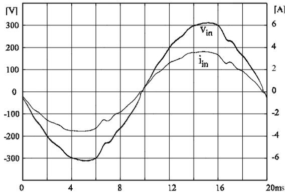
Fig. 11 - Line voltage and current waveforms.
