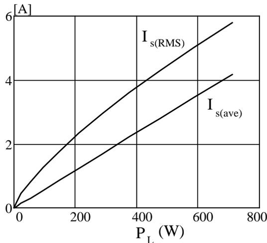
Figure 7. Average and RMS current through switch S.
