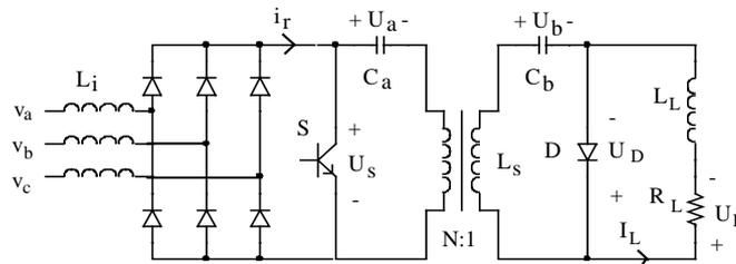
Fig. 1. Isolated Cuk converter with inductive load.
