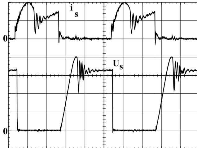
Fig. 9. Top trace: Transistor current (2A/div.)
