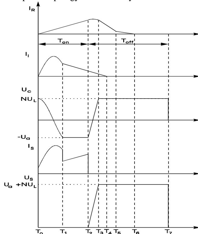
Fig. 4. Main converter waveforms: ideal case (without transformer leakage inductance)
