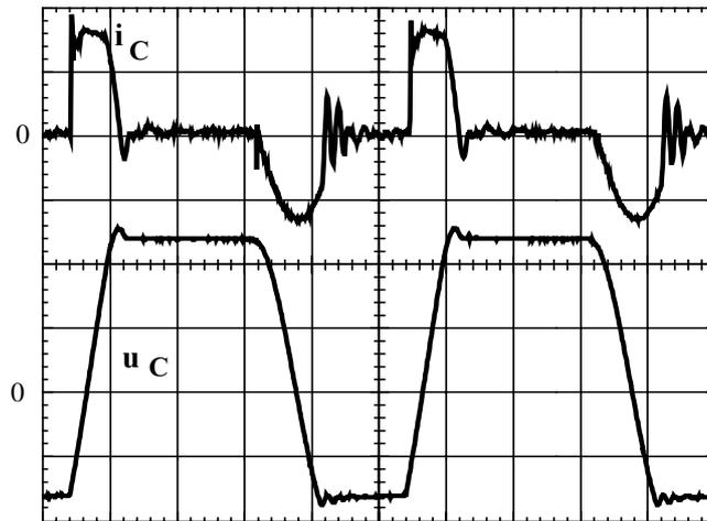
Fig. 10. Capacitor  $C_c$  current (top) (5A/div) and voltage (bottom) (200V/div) Horiz.: 4 $\mu$ s/div
