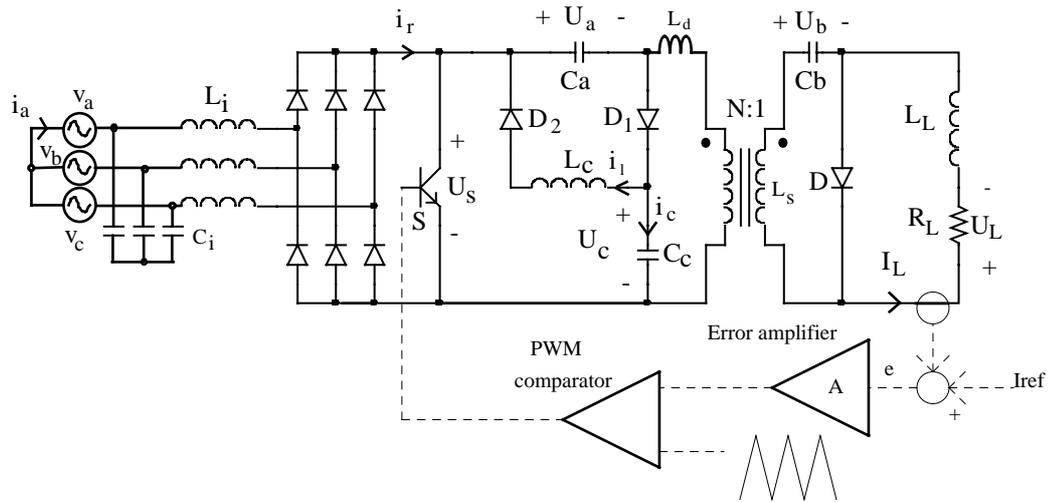
Fig. 3. Proposed topology with auxiliary circuit for soft-turn-off
