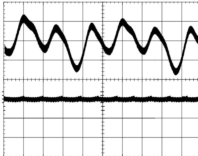
Fig. 11. Output current ripple (20 mA/div)
