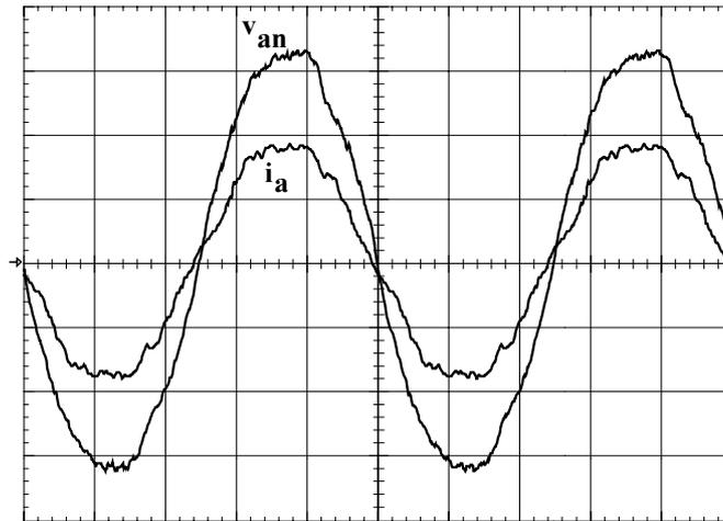
Fig. 12. Line voltage (50V/div) and current (1A/div) Horz.: 4ms/div
