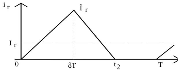
Fig. 2. Input current waveform
