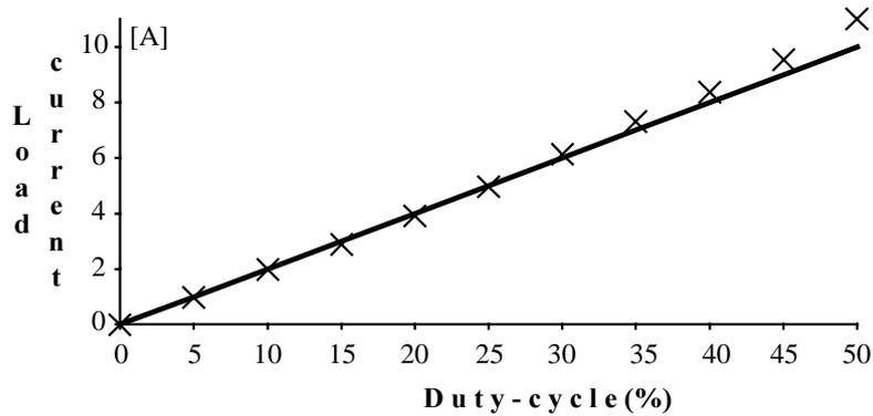
Fig. 6 Static characteristic of the converter
