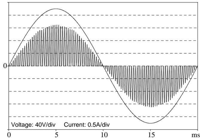
Fig. 8. Simulated input phase voltage and current (unfiltered)
