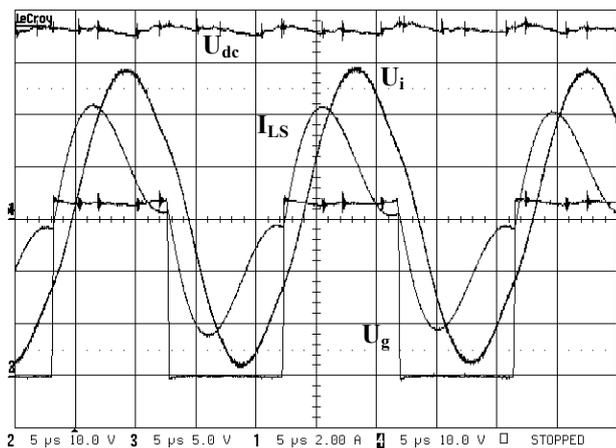
Fig. 7 - Typical converter waveforms at nominal output power for a seven lamp LCD. From top to bottom: SEPIC output voltage  $U_{dc}$  (5 V/div), PZT input voltage  $U_i$  (5 V/div, almost sinusoidal), inverter output current  $I_{LS}$  (2 A/div), inverter output voltage  $U_g$  (10 V/div). Timebase is 5  $\mu$ s/div.
