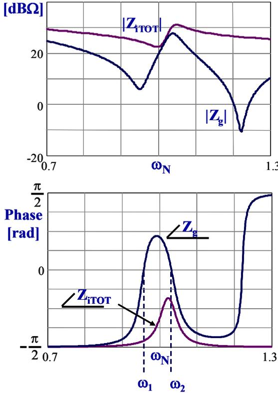
Fig. 3 – Magnitude and phase of the inverter load impedance ( $Z_g$ ) and of four parallel connected transformer input impedance ( $Z_{TOT}$ ). The frequency axis is normalized to the series resonance frequency ( $1/\sqrt{LC}$ ) of the model in Fig. 2. Soft switching is guaranteed between  $\omega_1$  and  $\omega_2$ .
