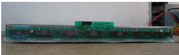
Fig. 6 - Piezoelectric transformers PCB. The board is located at the bottom of the LCD display.
