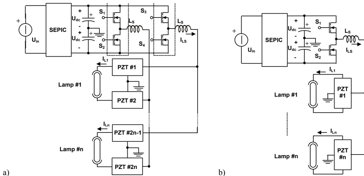
Fig. 1 –Schematic of the proposed power supply: a) single ended transformers; b) balanced output transformers.
