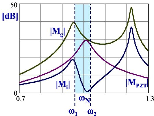
Fig. 4 – Magnitude of piezoelectric transformer voltage gain ( $M_{PZT}$ ), of the voltage gain from inverter output to transformer input ( $M_i$ ) and of the overall voltage gain from inverter output to transformer output ( $M_g$ ). The frequency axis is normalized to the series resonance frequency ( $1/\sqrt{LC}$ ) of the model in Fig. 2.
