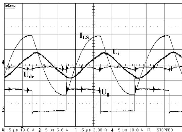
Fig. 8 - Typical converter waveforms at reduced output power (maximum dimming) for a seven lamp LCD. From top to bottom: inverter output current  $I_{LS}$  (2 A/div), PZT input voltage  $U_i$  (5 V/div), SEPIC output voltage  $U_{dc}$  (5 V/div), inverter output voltage  $U_g$  (10 V/div). Timebase is 5  $\mu$ s/div.
