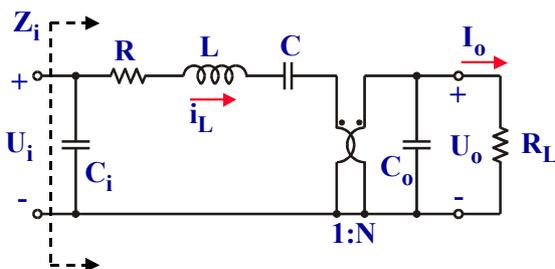
Fig. 2 – Equivalent electrical model of the Rosen type piezoelectric transformer.
