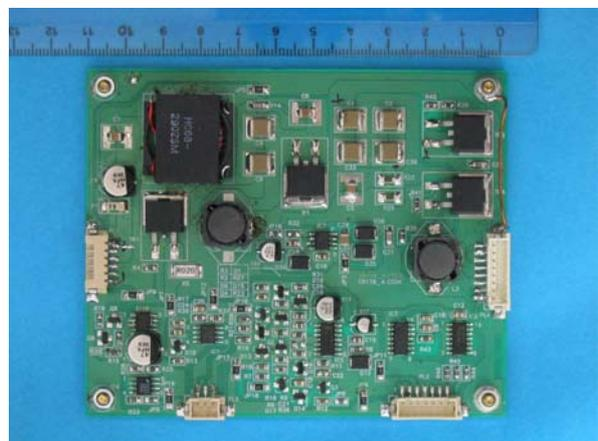
Fig. 5 - PCB of the power supply.
