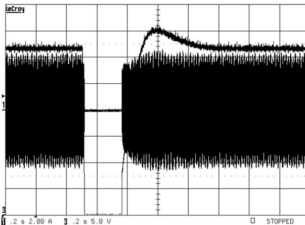
Fig. 9 - Typical start-up waveforms. From top to bottom: SEPIC output voltage  $U_{dc}$  (5 V/div), inverter output current (2 A/div). Timebase is 200 ms/div.
