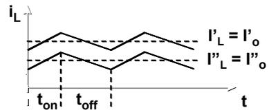
$$\Delta I'_L = \Delta I''_L \quad \Delta I_L = f(U_o) = \frac{U_i \delta (1 - \delta)}{f_s L}$$
