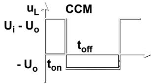
$$(U_i - U_{oCCM}) t_{on} = U_{oCCM} t_{off}$$
