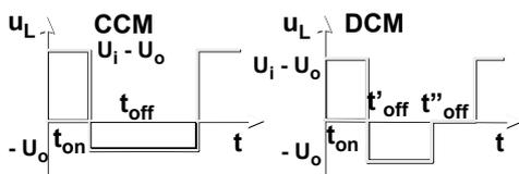
$$U_i t_{on} = U_{oCCM} T_s \quad U_i t_{on} = U_{oDCM} (t_{on} + t'_{off})$$
