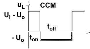
$$(U_i - U_{oCCM}) t_{on} = U_{oCCM} t_{off}$$
