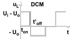
$$(U_i - U_{oDCM}) t_{on} = U_{oDCM} t'_{off}$$
