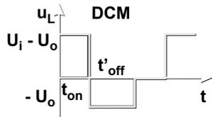
$$(U_i - U_{oDCM}) t_{on} = U_{oDCM} t'_{off}$$
