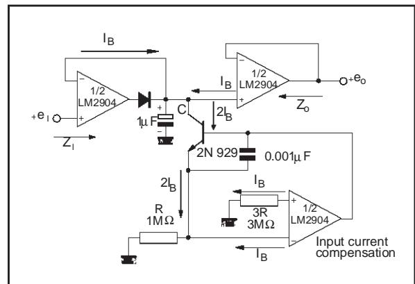
**USING SYMMETRICAL AMPLIFIERS TO REDUCE INPUT CURRENT**
