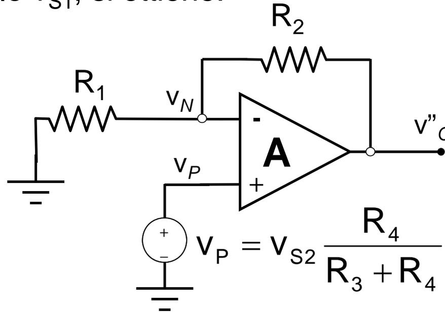
$$v''_O = v_{S2} \left( \frac{R_4}{R_3 + R_4} \right) \left( 1 + \frac{R_2}{R_1} \right)$$
