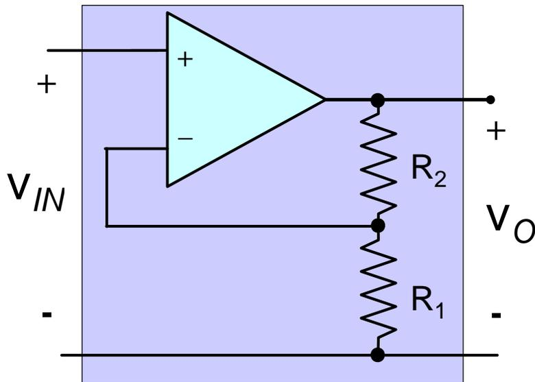
$$A_v = \frac{v_O}{v_{IN}} = \left( 1 + \frac{R_2}{R_1} \right)$$
