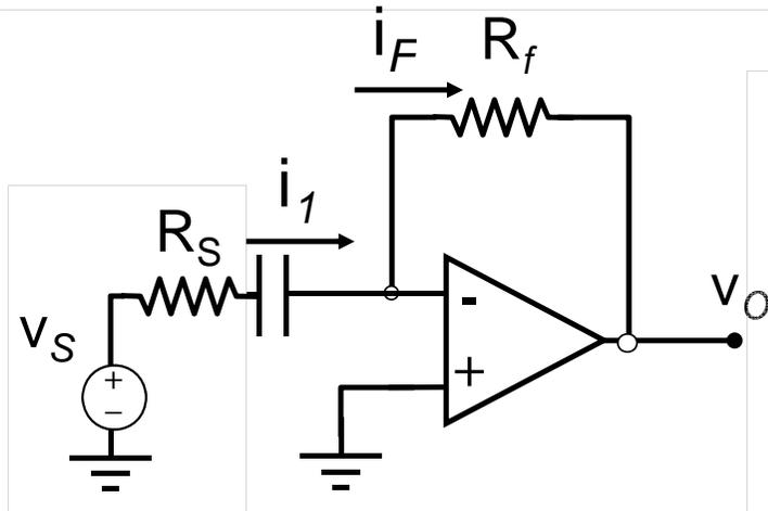
$$W(s) = -\frac{R_f}{R_s + \frac{1}{sC_1}} = -\frac{sR_f C_1}{1 + sR_s C_1}$$
