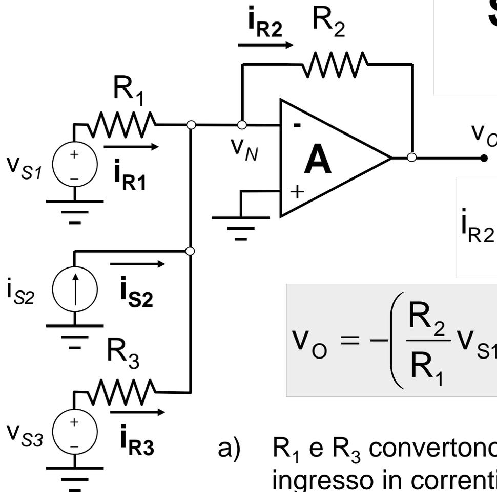
$$i_{R2} = \frac{v_{S1}}{R_1} + i_{S2} + \frac{v_{S3}}{R_3}$$
