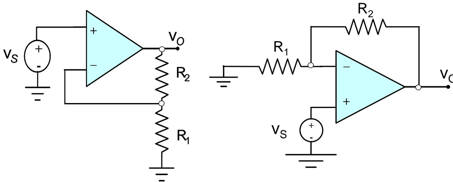
$$A = \frac{V_O}{V_S} = \left( 1 + \frac{R_2}{R_1} \right)$$
