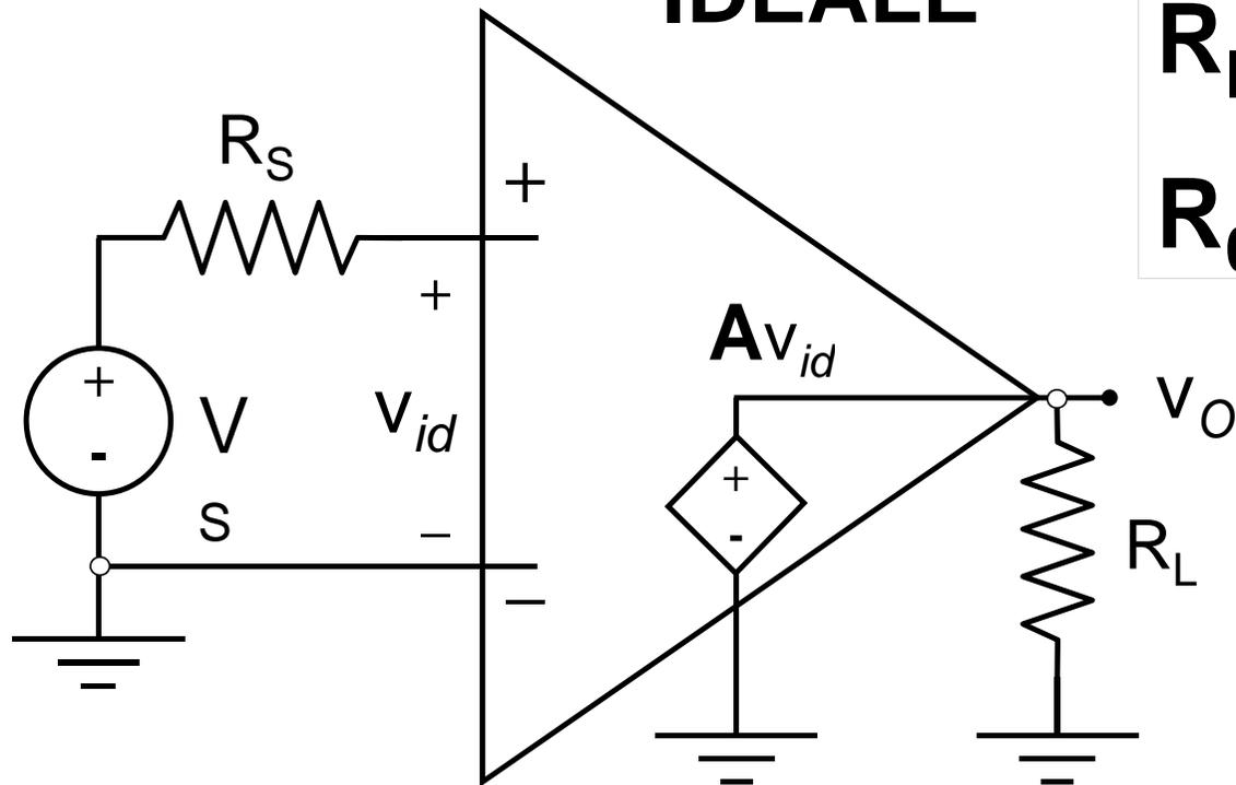
$$A_v = \frac{v_o}{v_s} = A \cdot \frac{R_{id}}{R_{id} + R_s} \cdot \frac{R_L}{R_L + R_0} = A$$
