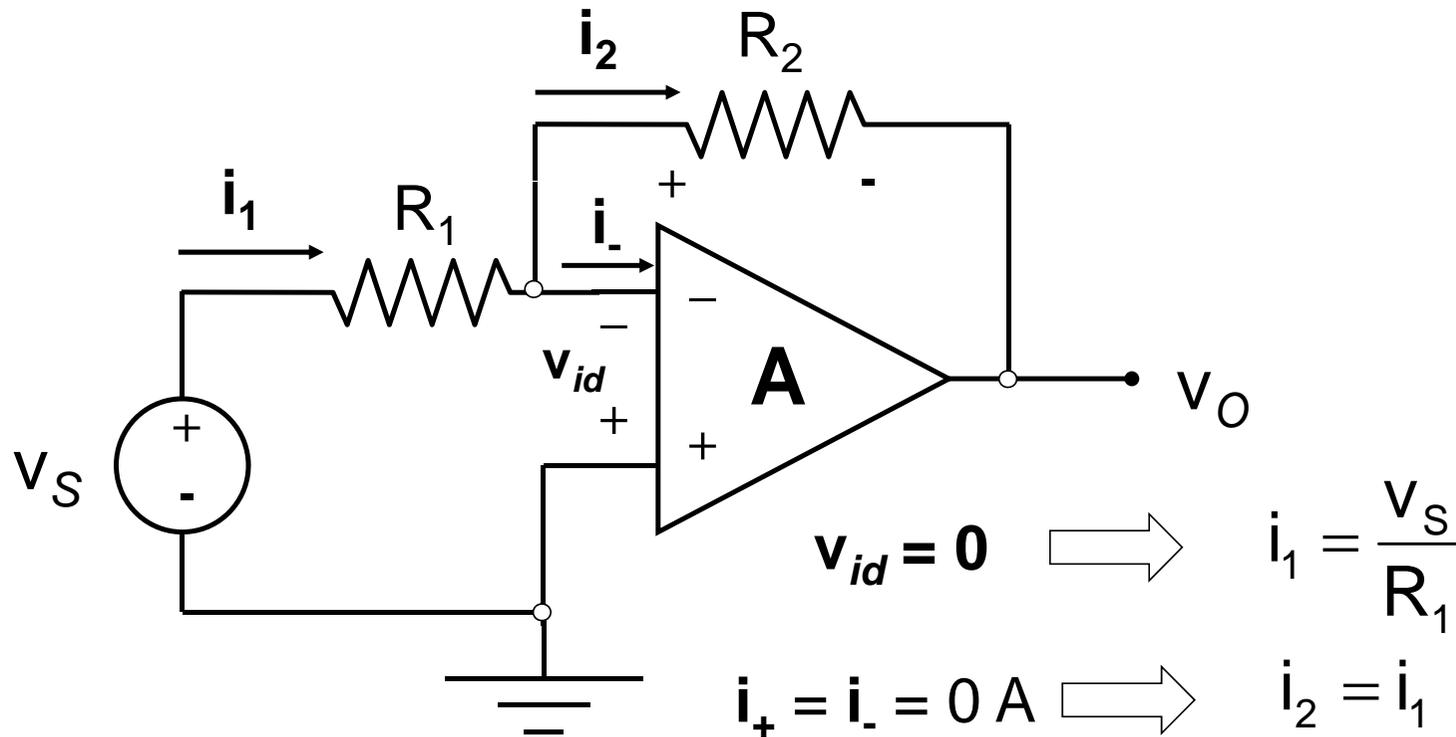
$$v_O = -R_2 i_2 = -\frac{R_2}{R_1} v_S$$
