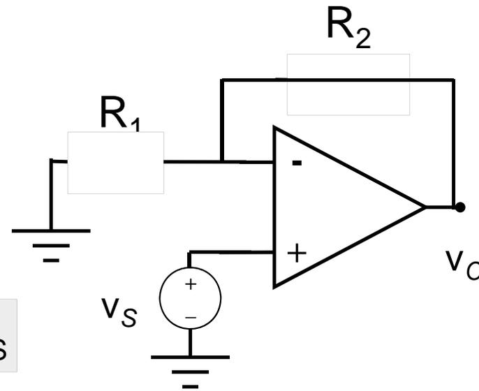
$$A_v = \frac{v_O}{v_{IN}} = \left( 1 + \frac{R_2}{R_1} \right)$$
