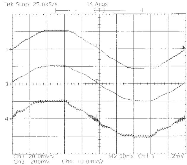
Fig. 12. Test conditions: no filter on the estimated line voltage;  $V_{dc} = 120$  V;  $\Delta L\% = 0$ ; time scale: 2 ms/div; rectifier mode; Upper trace: estimated line voltage (200 mV/div). Middle trace: line to neutral measured voltage (40 V/div). Lower trace: phase current (1 A/div).
