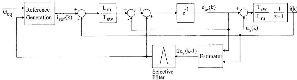
Fig. 6. Block diagram of the proposed control solution.
