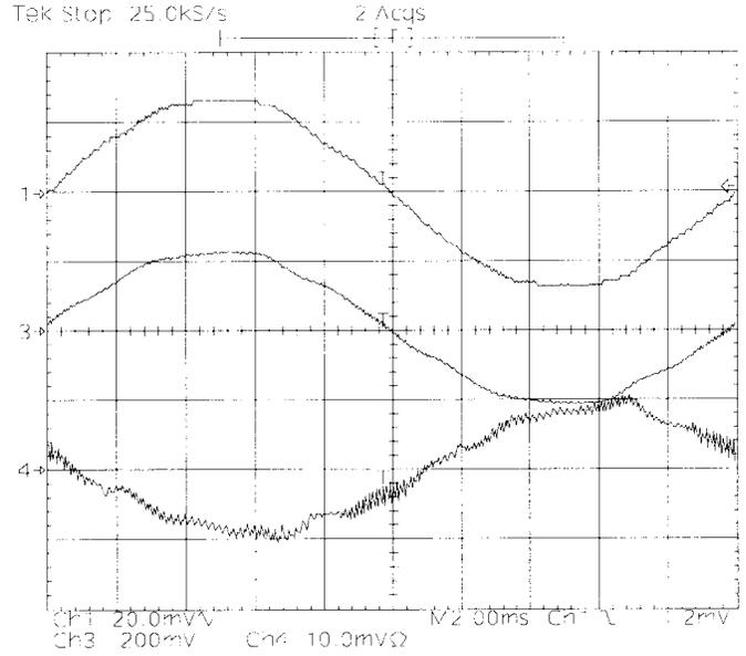
Fig. 15. Test conditions: no filter on the estimated line voltage;  $V_{dc} = 120$  V;  $\Delta L\% = 0$ ; time scale: 2 ms/div; generator mode. Upper trace: estimated line voltage (200 mV/div). Middle trace: line-to-neutral measured voltage (40 V/div). Lower trace: phase current (1 A/div).
