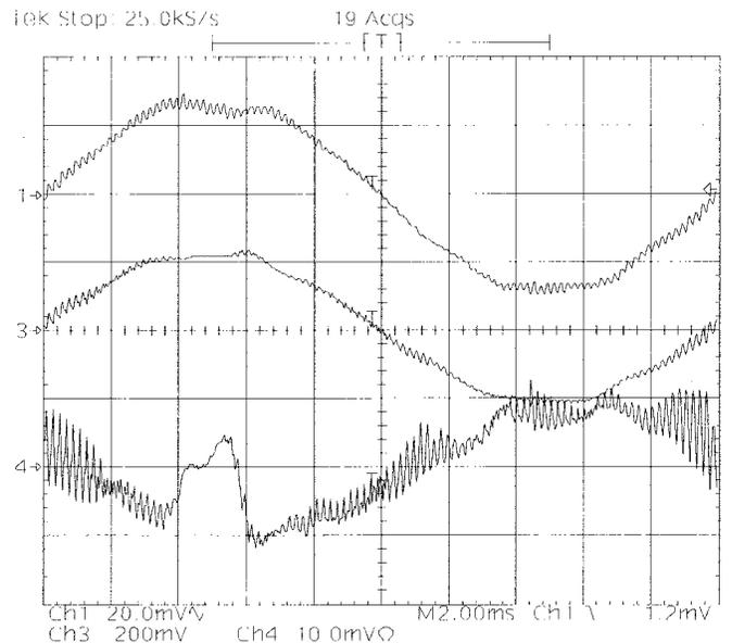
Fig. 16. Test conditions: no filter on the estimated line voltage;  $V_{dc} = 120$  V;  $\Delta L\% = 5\%$ ; time scale: 2 ms/div; generator mode. Upper trace: estimated line voltage (200 mV/div). Middle trace: line-to-neutral measured voltage (40 V/div). Lower trace: phase current (1 A/div).
