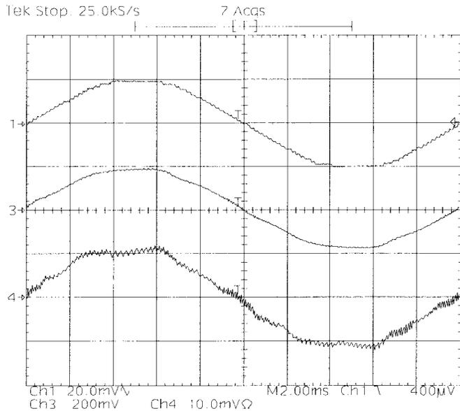
Fig. 17. Test condition: filter on the estimated line voltage both for reference and dead-beat calculations;  $V_{dc} = 120$  V;  $\Delta L\% = 30\%$ ; time scale: 2 ms/div; rectifier mode. Upper trace: estimated line voltage (200 mV/div). Middle trace: line to neutral measured voltage (40 V/div). Lower trace: phase current (1 A/div).
