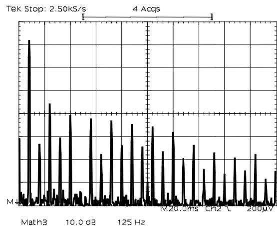
Fig. 7 – Input current  $i_g$  spectrum (10 dB/div). Horizontal: 125 Hz/div
