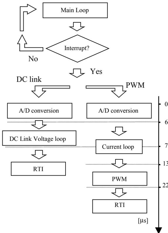
Fig. 5 – Flow chart of the control program
