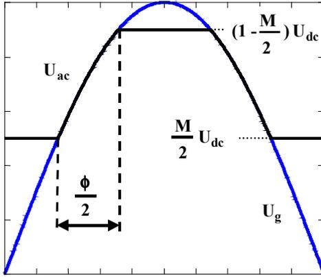
Fig. 2 – Converter's average input voltage  $U_{ac}$  and line voltage  $U_g$ . Current control is possible only within an angle  $\phi$  of the line voltage half-period.
