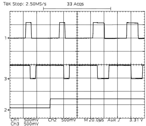
Fig. 4 – Operation of the digital PWM modulator.
