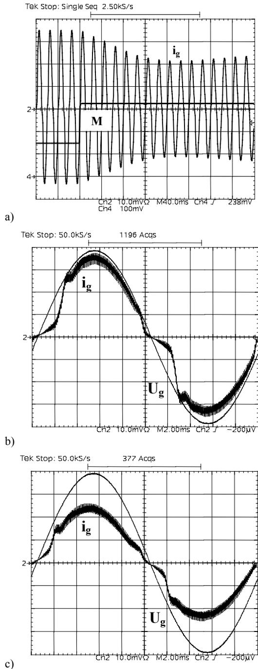
Fig. 8 – a) Transient in the M parameter from 0.5 to 0.4. Input current  $i_g$  (2 A/div) and M signal. Horizontal: 40 ms/div
