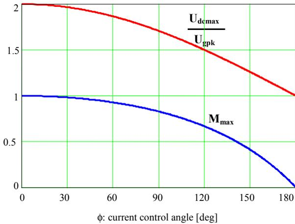
Fig. 3 – Upper trace: ratio between  $U_{dc}$  and line voltage peak value  $U_{gpik}$  as a function of the line control angle. Lower trace: maximum modulation index  $M_{max}$  as a function of the line control angle.
