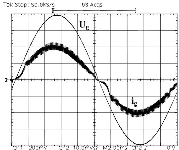
Fig. 6 – Input voltage  $U_g$  (40 V/div) and current  $i_g$  (2 A/div). Horizontal: 2 ms/div
