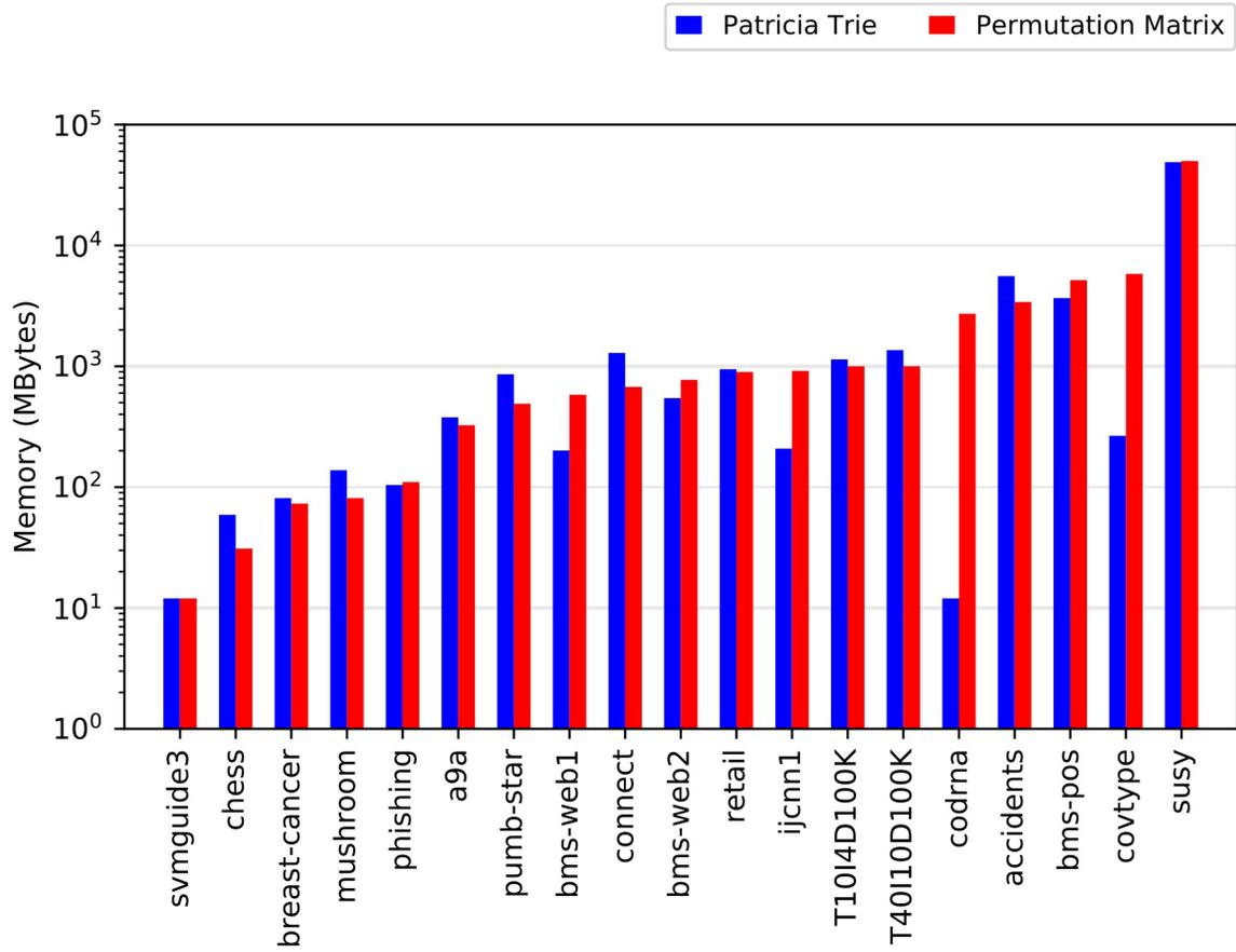
Figure 3-3: Memory requirement for permuted class labels using PatriciaTrie and permutation matrix.
