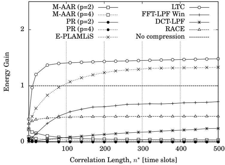
Fig. 6. Maximum Energy Gain vs Correlation Length  $n^*$  for a single-hop scenario.
