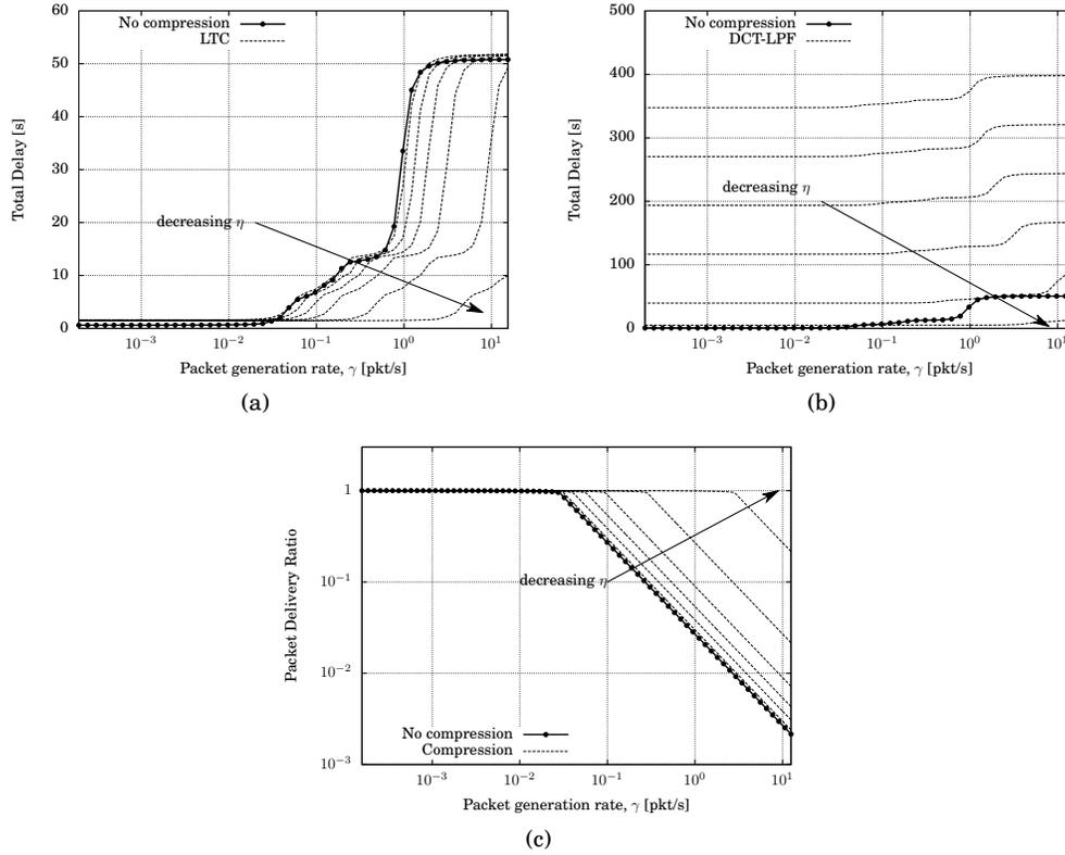
Fig. 11. Total Delay [s] vs packet generation rate  $\gamma$  at the lowest level for: (a) LTC; (b) DCT-LPF. (c) Packet Delivery Ratio vs packet generation rate  $\gamma$  at the lowest level.
