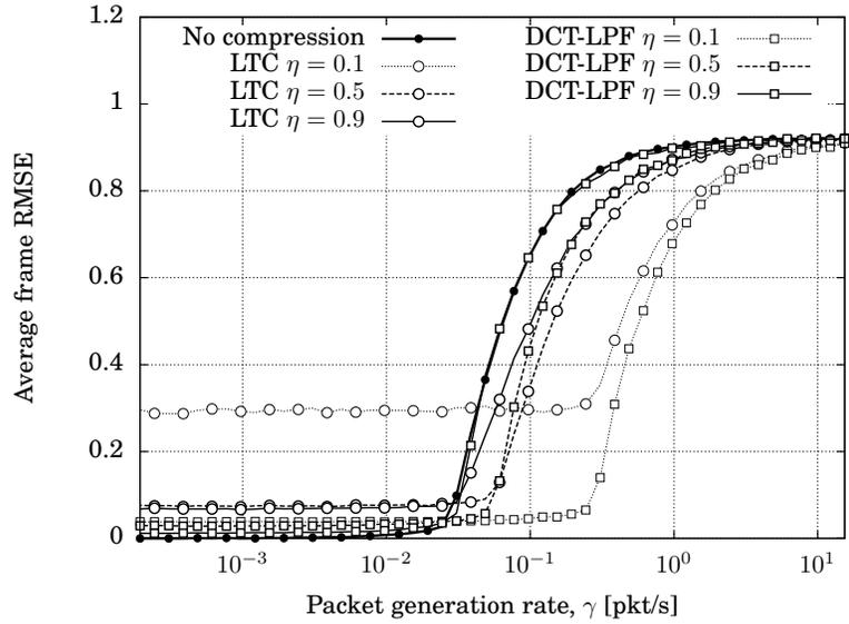
Fig. 13. Average frame RMSE vs packet generation rate  $\gamma$  for an input signal with  $n^* = 290$ .
