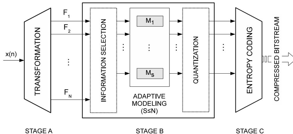
Fig. 1. General lossy compression diagram.
