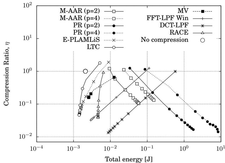
Fig. 5. Compression Ratio  $\eta$  vs Total Energy Consumption: comparison among lossy compression schemes.
