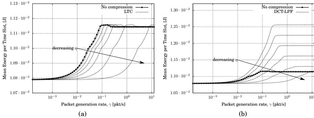
Fig. 12. Mean energy per time slot [J] vs packet generation rate  $\gamma$  at the lowest level: (a) LTC; (b) DCT-LPF.
