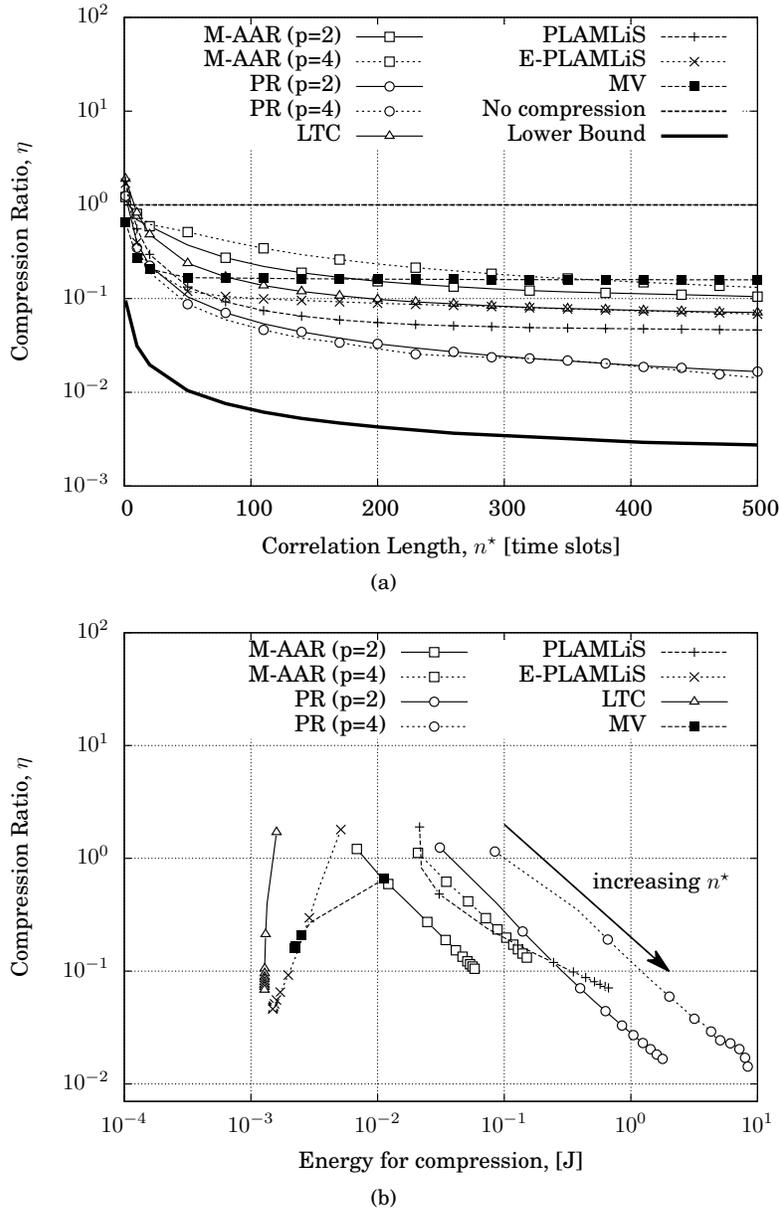
Fig. 3. (a)  $\eta$  vs Correlation Length  $n^*$  and (b)  $\eta$  vs Energy consumption for compression for the Adaptive Modeling methods for fixed  $\varepsilon = 4\sigma_{\text{noise}}$ .
